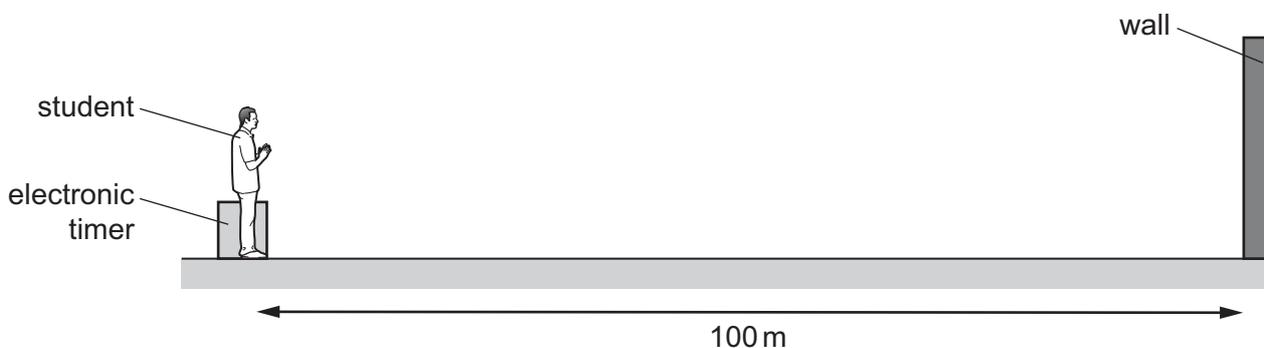
An electronic timer next to the student detects the echo of the sound 0.60 s after it is made.
